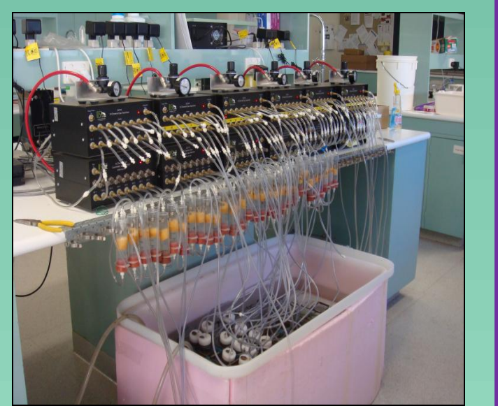
Respirometer used for measuring heterotrophic soil respiration in the laboratory at 20°C.
