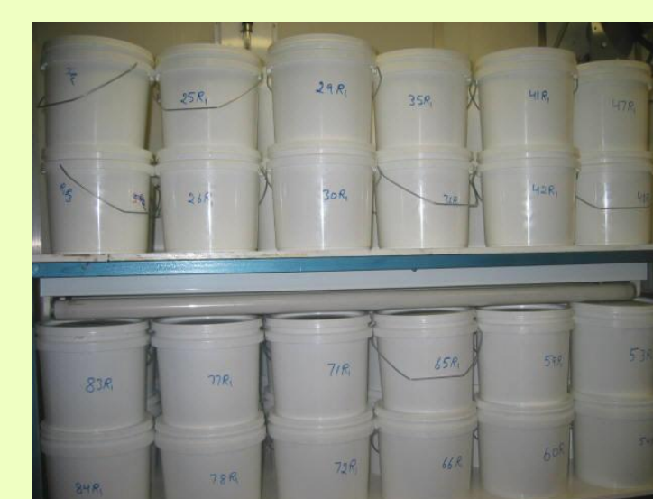
Sealed buckets used for the biochar-C turnover experiment. The NaOH solution in the bucket traps the \text{CO}_2 released during biochar decomposition.
